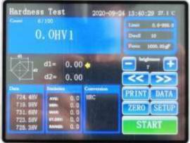
5.6" multiple Functions Touch Screen with Hardness Conversation Functions
