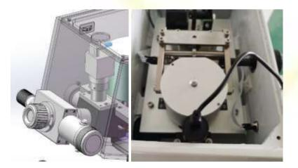
Double optical path design. Both eyepiece and CCD camera path can work at same time. No need switch optical path.
