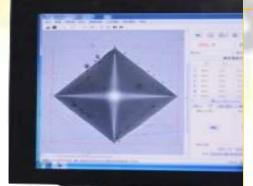
Advanced HV / HK Micro Hardness Indentation Measurement and Analysis system support automatic work mode and manual work mode. And can generate test report in word / Excel format directly, report data including indentation image, hardness value, test force, dwell time, hardness curve, indentation depth, etc.
