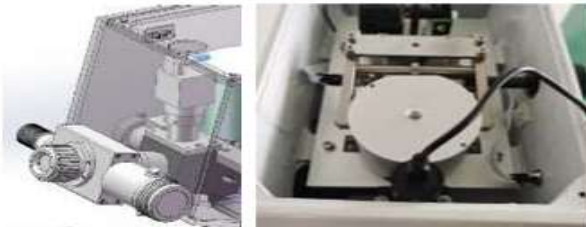
Precision Manual measuring eyepiece (10X) Resolution 0.5µm
