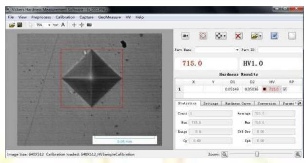
Software support automatic measurement & manual measurement can generate test report automatically in word / Excel format, including hardness value, test force, indentation image and hardness curve, etc.
