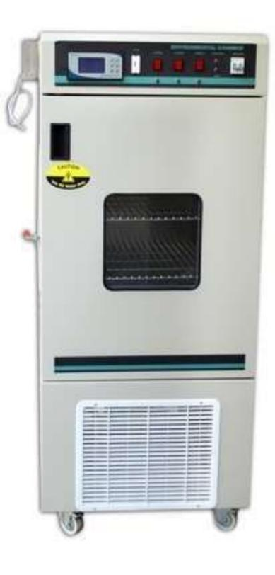
HSMLE humidity Chamber is a unique test cabinet designed to create temperature and relative humidity inside the chamber to detect the change in the physical characteristics of material & to ascertain the actual working life of the testing device.
