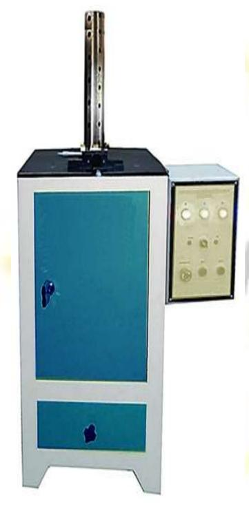
Our motorized broaching machine is a selfcontained floor-mounted unit, specially designed for cutting 'V' and 'U' notches in standard 10mm square, sub-size and 0.45" diameter specimens. Our V/U Notch Broaching Machines are suitable for ferrous & non-ferrous material for sample preparation of 'V' or 'U' notches for Impact Testing Machines.
